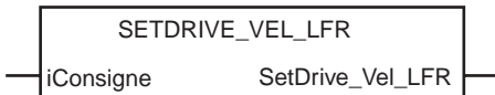
Example of a function block: sending the speed reference to the drive
