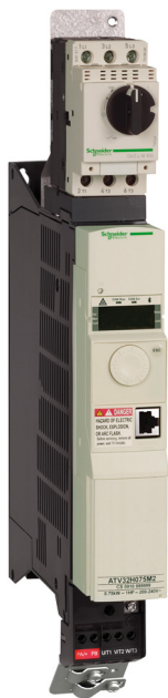
GV2/ATV32 direct mounting: GV2L08 + (VW3A9921 + GV2AF4) (3) + ATV32H075N4
